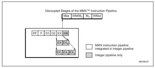
Instruction parsing is decoupled from the instruction decoding by means of an instruction FIFO, which is situated between the F and D1 (Decode 1) stages. The FIFO has slots for up to four instructions. This FIFO is transparent, it does not add additional latency when it is empty.
